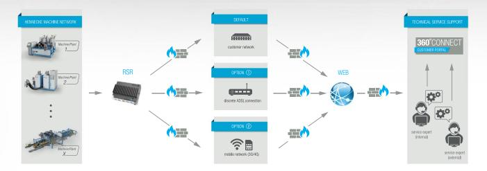
The necessary technology based on the Process Data Acquisition (PDA) software is already installed in each Hennecke plant with PC terminal. For machines and systems in which only PLC automation is being used, the data connection for remote service is established over a Remote Service Router (RSR)\*. Both solutions impose **minimum requirements on your firewall** because only a single communication port is used in the entire communication process:
