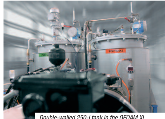
Double-walled 250-l tank in the QFOAM XL
