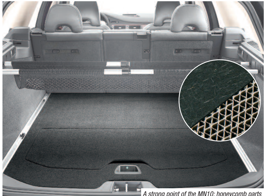
A strong point of the MN10: honeycomb parts
