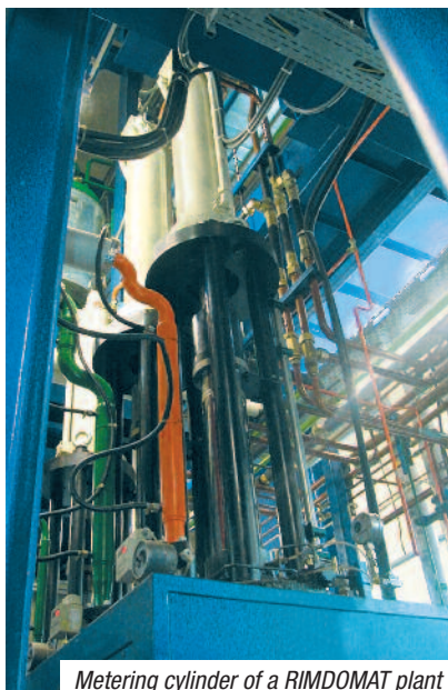
Metering cylinder of a RIMDOMAT plant
