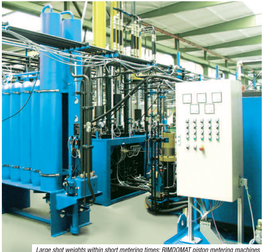
Large shot weights within short metering times: RIMDOMAT piston metering machines
