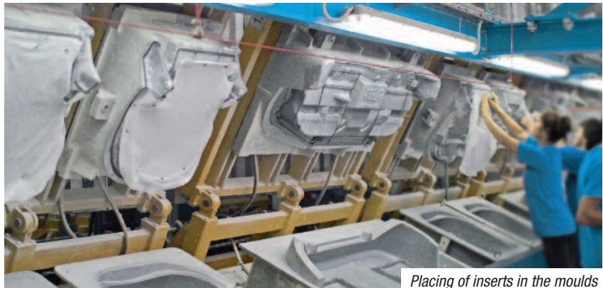
Placing of inserts in the moulds
