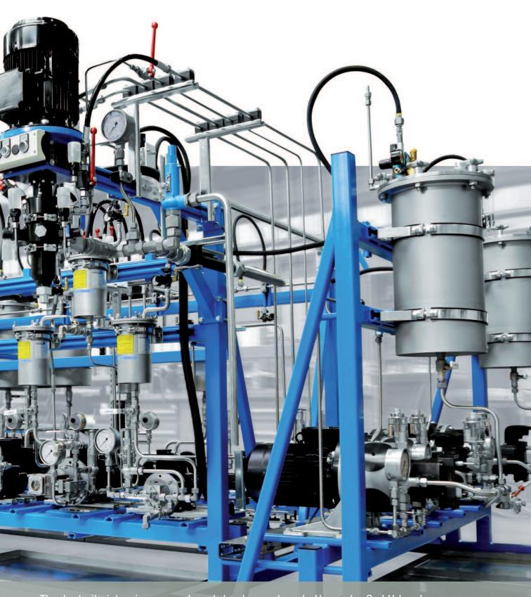
Thanks to its intensive research and development work, Hennecke GmbH has become a leading supplier of PU processing technology. This especially applies to machines and systems for manufacturing high-quality slabstock foams. To help producers and raw material suppliers develop innovative formulations and carry out production equivalent trials with top quality results even for small volumes, Hennecke offers a special laboratory plant.
