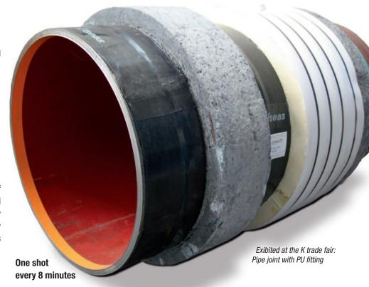
The steel pipes are automatically welded during the pipe-laying process. Shrink tubing is then pulled over the weld site and the interruption of the concrete sheathing is sealed with a sleeve. The hollow space that is formed is then filled with Elastopor H. Up to 45 (!) kgs can fit into such a fitting. Some 200,000 fittings have to be filled, meaning that HK machines are performing one shot every 8 minutes, 24 hours a day and 7 days a week until the pipe laying operation is over.
