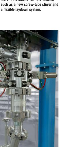
New laydown system with flexible outlet geometry
