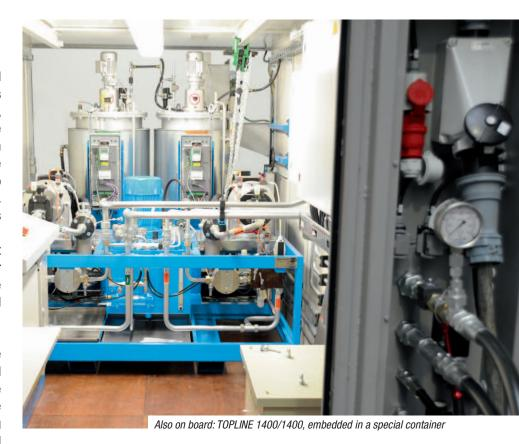
At the last "K" trade fair Allseas approached Hennecke with an enquiry about a special machine that had to be mobile so that it could be fitted onto a ship. It also had to have an output of over 3 kg/s and be suited to raw materials systems with mixing ratios of 50 to 100 to 150. Moreover, it had to have its own cooling circuit for ambient temperatures of between minus 30 and plus 50 degrees Celsius.
