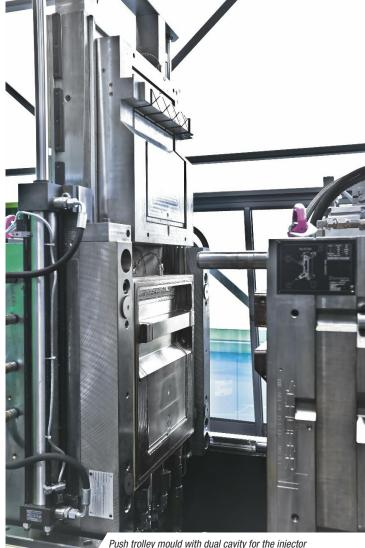
Push trolley mould with dual cavity for the injector side and single cavity for the lower mould
