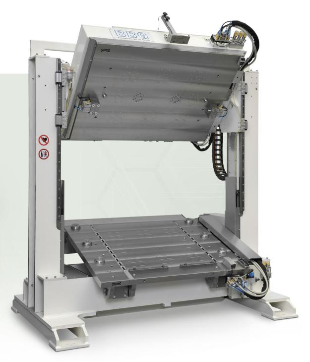
End-to-end solution for encapsulating vehicle glass: GlassLine metering machine and BBG mould carrier system BFT-PV7
