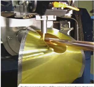
Continuous production of Flex pipes: laminar foam discharge onto the inner PE film using an MT-8 high-pressure mixhead with constant pressure injectors
