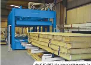
PANELFOAMER with hydraulic lifting device for transporting the building components
