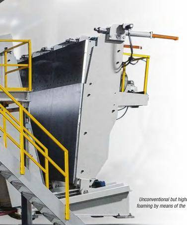
Unconventional but highly efficient: foaming by means of the "free-rising foam method" using the A-frame double press
