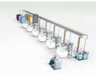
For production on a grand scale: addition of further isocyanate units (I.) and extension with ring lines for high material throughput (r.)
